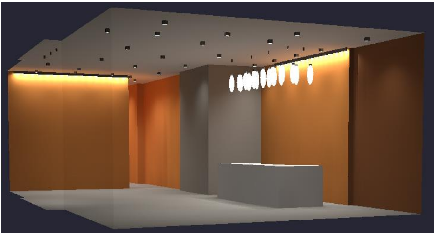
Figure 35: Rendering of the lobby and reception areas is displayed. A combination of fluorescent and CFL downlights, wall washers and pendants combine to produce an acceptable lighting scheme for the LED to fluorescent redesign. (Courtesy AGi32-16.7)
