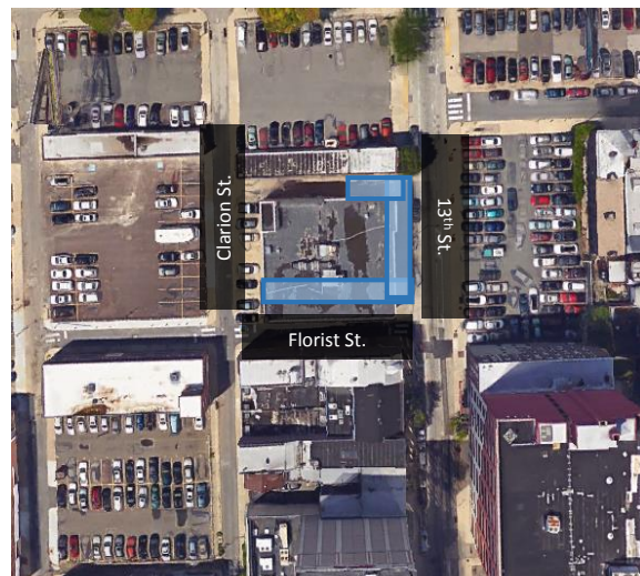
Figure 10: Existing exterior walls to remain after demolition (Courtesy Google Maps)
